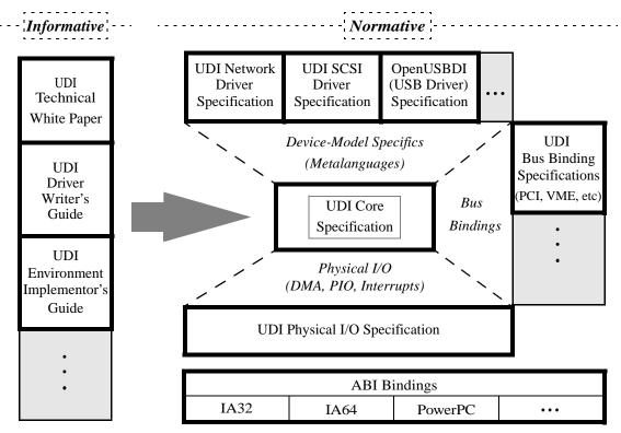
This picture is intended to show the types of books in the UDI document set: driver-type specific specifications, bus bindings, ABI bindings, physical I/O interfaces, etc., all of which are centrally supported by the UDI Core Specification. Not all of the books mentioned in this figure will be available coincident with the publishing of the UDI Core Specification.
