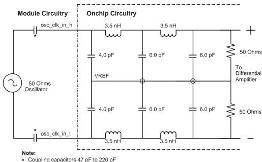
Figure 9–1 osc\_clk\_in\_h,l Input Network and Terminations
