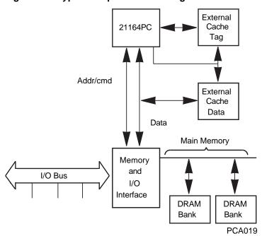
Figure 2–4 Typical Uniprocessor Configuration
