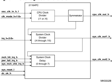
Figure 4-4 Clock Signals and Functions
