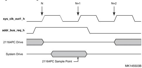
To pass control of the command/address bus back to the 21164PC, the system should turn off its drivers during a sysclk cycle and deassert addr bus req h. The 21164PC does not sample the state of the bus if **addr bus req h** is deasserted. The 21164PC drives the command/address bus at the rising edge of sysclk N+2.
