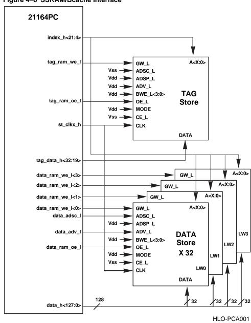
Figure 4-8 SSRAM/Bcache Interface
