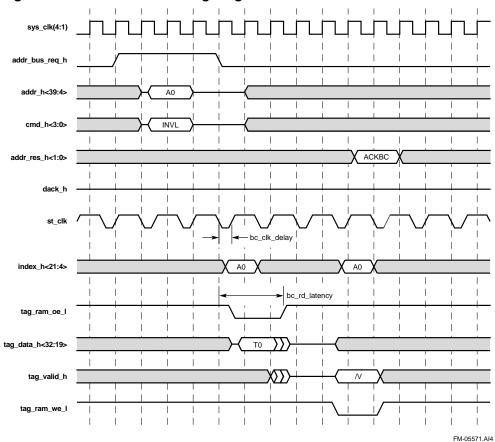
Figure 4-20 INVALIDATE Timing Diagram - Bcache Hit
