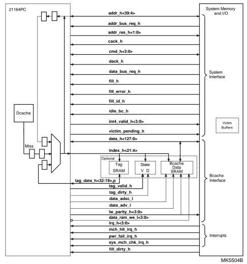
Figure 4–1 21164PC System/Bcache Interface
