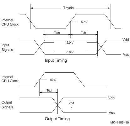
Figure 9–3 Input/Output Pin Timing
