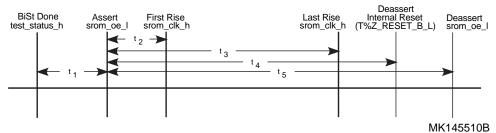
Figure 9–7 SROM Load Timing Event—Timeline
