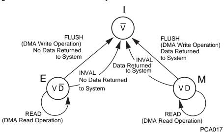
Figure 4–7 Flush-Based Protocol System/Bus States
