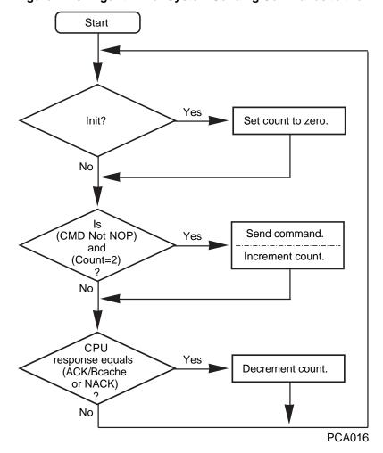
Figure 4–18 Algorithm for System Sending Commands to the 21164PC
