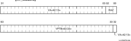
Figure 5–7 shows the IFAULT\_VA\_FORM register format in NT mode.
