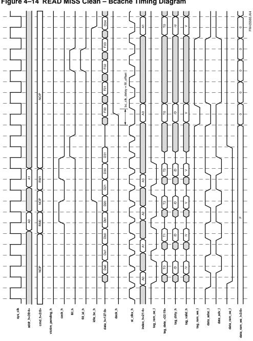
Figure 4–14 READ MISS Clean – Bcache Timing Diagram
