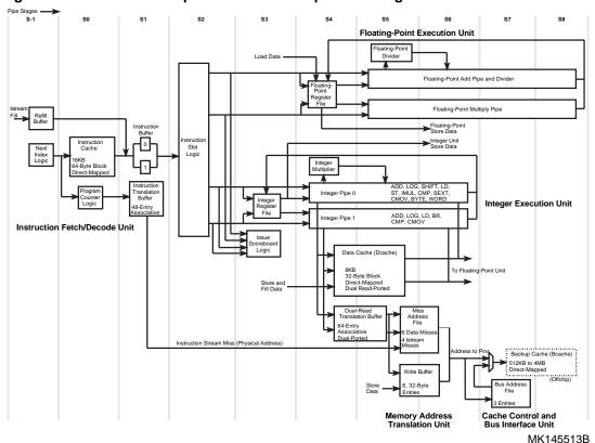
Figure 2-1 21164PC Microprocessor Block/Pipe Flow Diagram
