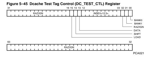
Table 5–22 Dcache Test Tag Control Register Fields
