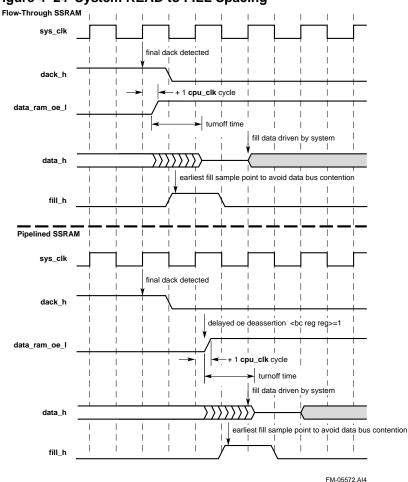
Figure 4-24 System READ to FILL Spacing
