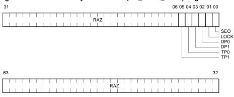
Figure 5–37 Dcache Parity Error Status (DC\_PERR\_STAT) Register
