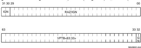
Figure 5–9 shows the IVPTBR register format in NT mode.
