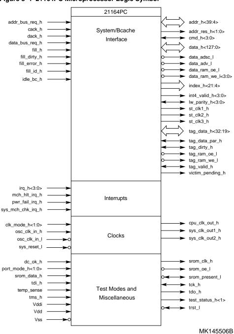
Figure 3-1 21164PC Microprocessor Logic Symbol
